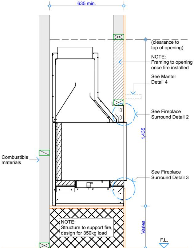
Cross Section - Fire Insert at Floor Level
