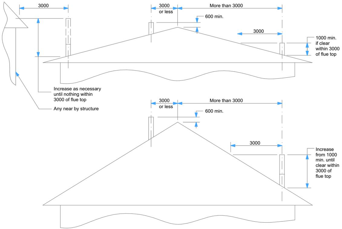
**Minimum Height of Flue System Exit**
