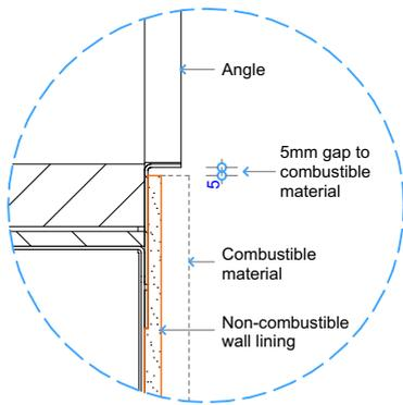
Detail 3 - Bottom of Fire to Floor
