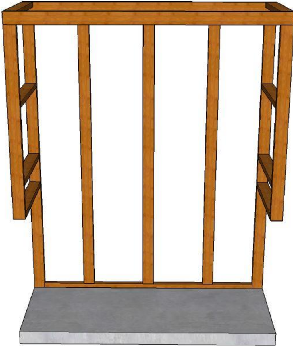
The starting point: Timber frame with concrete hearth.
