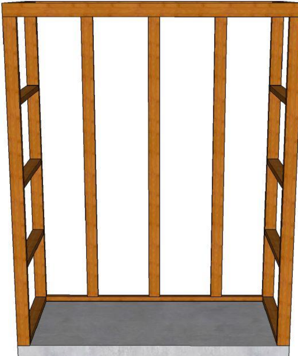
The starting point: Timber frame with concrete hearth.
