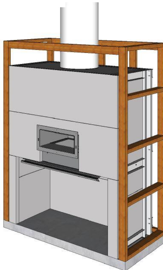
Front AAC panels complete.
