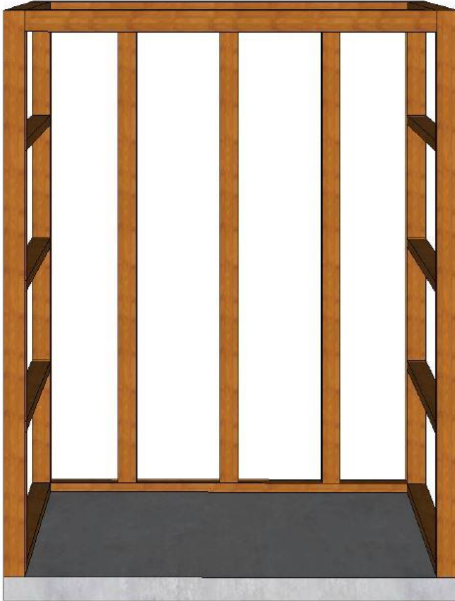
The starting point: Timber frame with concrete hearth.
