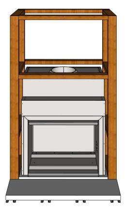
2. With a minimum of two people, slide the firebox and outer cavity box into position.
