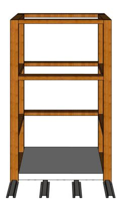
2. Fix rear AAC panel to steel supporting brackets. Countersink 2 x 5mm 80mm long steel screws per bracket.
