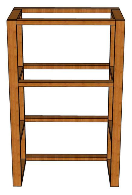
The starting point: Timber frame. Note: Timber lintel to suit opening must be fitted after appliance has been fixed into position.
