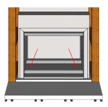
3. Fix the fire box through the AAC panel and into the AAC supporting brackets. 2 x 5mm x 120mm long self-drilling steel fixings.
