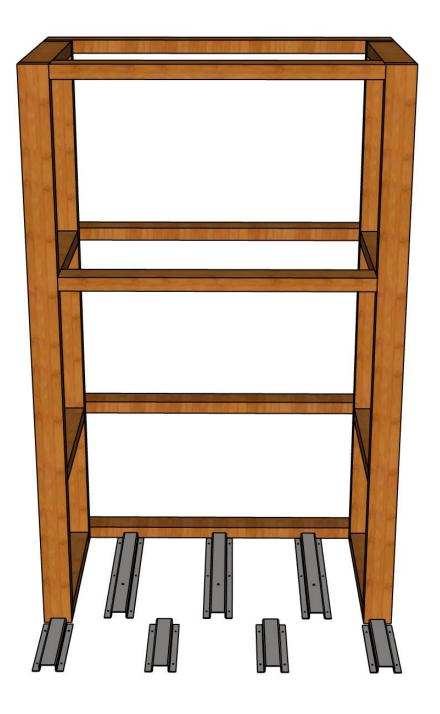
Fix the AAC supporting brackets into position in accordance with technical specifications (example shown). Rear brackets have 6 x fixing holes each and the front brackets have 4 x fixings holes each. 5mm screws/bolts.
