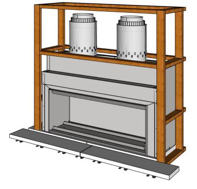
1. Run the flue transition. The flue runs into the firebox. The inner casing runs into the outer cavity box. The outer casing finishes 25mm above the outer cavity box.
