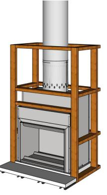
3. Complete the rest of the timber lintel framing in accordance with appropriate technical specifications.
