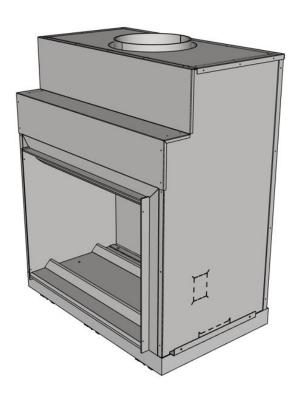
5. Lower the outer cavity box over the firebox.
