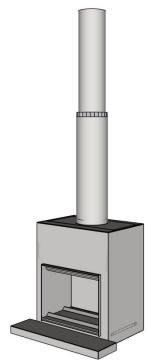
2. Run the first casing. The crimped end is at the top. The casing fits over the spigot on the outer rear panel. Position the seam in the casing to the least viewed direction of the appliance.
