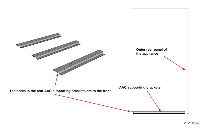
The back of the AAC supporting brackets are located and fixed into position 45mm forward of the rear panel of the appliance.
