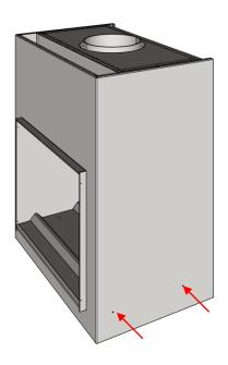
7. The outer panel is fixed to the brackets with 2 x 5mm countersunk cap screws at each side.
