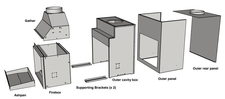
1. Disassemble the appliance by following the process below.
