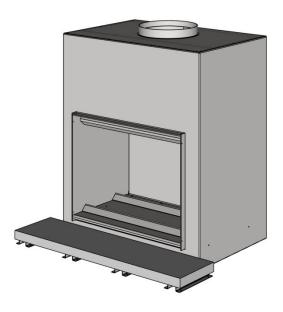
2. Fix hearth AAC panel to steel supporting brackets. Countersink 2 x 5mm x 65mm long steel screws per bracket.
