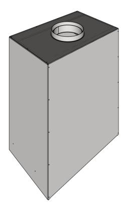
8. Fit the outer rear panel to the outer panel. 20 x 5mm countersunk cap screws.
