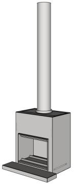
1. Run the 2 x flues. The crimped end runs into the firebox spigot.
