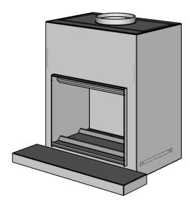
3. Finish hearth AAC panel in accordance with technical specifications (box-folded steel hearth cover example shown).
