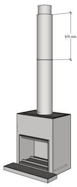
3. Run the second casing. No crimped The casing fits over the crimped end on the first casing.
