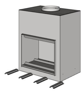
Fix the AAC hearth supporting brackets into position in accordance with technical specifications. The hearth brackets have 4 x fixings holes each. 6mm screws/bolts.
