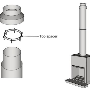
4. Fit the top spacer over the flue and into the casing.
