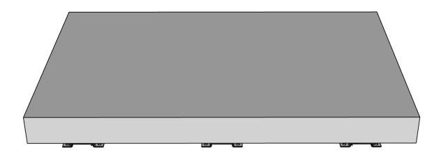
1. Fix base AAC panel to steel supporting brackets. Countersink 2 x 5mm 80mm long steel screws per bracket.
