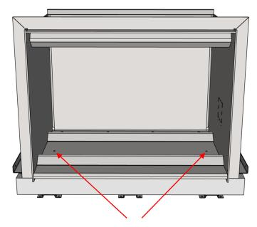
3. Fix the fire box through the AAC panel and into the AAC supporting brackets. 2 x 5mm x 120mm long self-drilling steel fixings.
