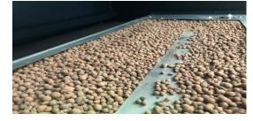
If LPG is being used, lightly cover burner slots in a thin layer of clay balls by adding at back of burner tray and gently sweeping forward.
