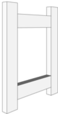
Step 1: Timber framing Set-up timber framing to suit wall cowl.
