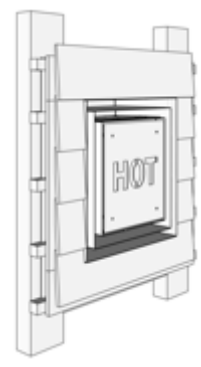
Step 4: Complete wall cladding Fit wall cladding in accordance with NZBC
