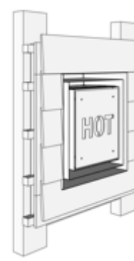
Step 4: Complete wall cladding Fit wall cladding in accordance with NZBC
