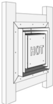
Step 2: Fit wall cowl into position Fix wall cowl into position through the angle surround.
