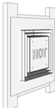
Step 3: Flash wall cowl Fit flashing in accordance with NZBC.
