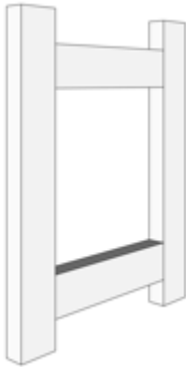
Step 1: Timber framing Set-up timber framing to suit wall cowl.
